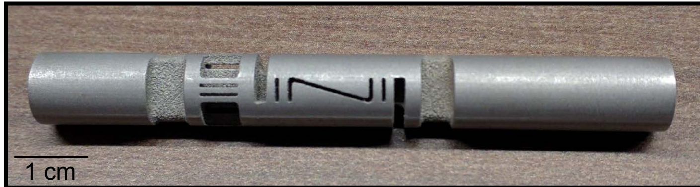
AM force balance produced by Morris Technologies*.
