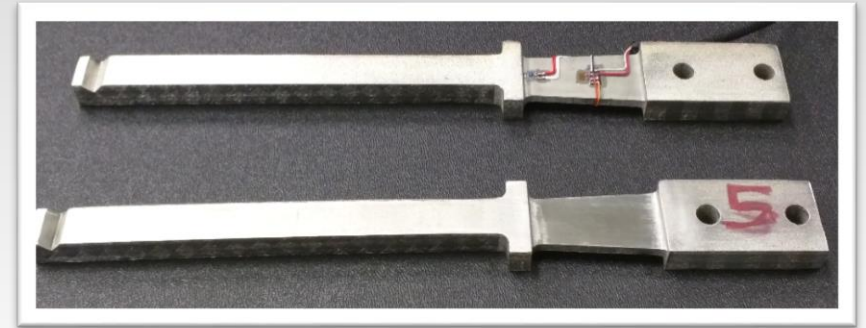
Two AM cantilever test beams.
