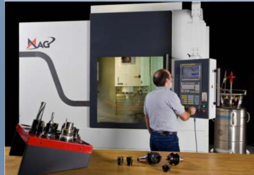
Cryogenic Machining – Technology Developed at Creare Transitioned to F-35 Titanium Part Machining
