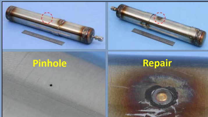
High-Speed, Additive Friction Stir Processing – Repair of Damage to Navy Ship Fuel System Piping and Navy Rotorcraft Components
