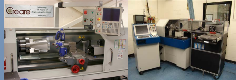
Vertical Machining Center: Lathe and Precision Machine Tool Equipped With Cryogenic Machining, On-Machine Measurement, Laser-Assist
